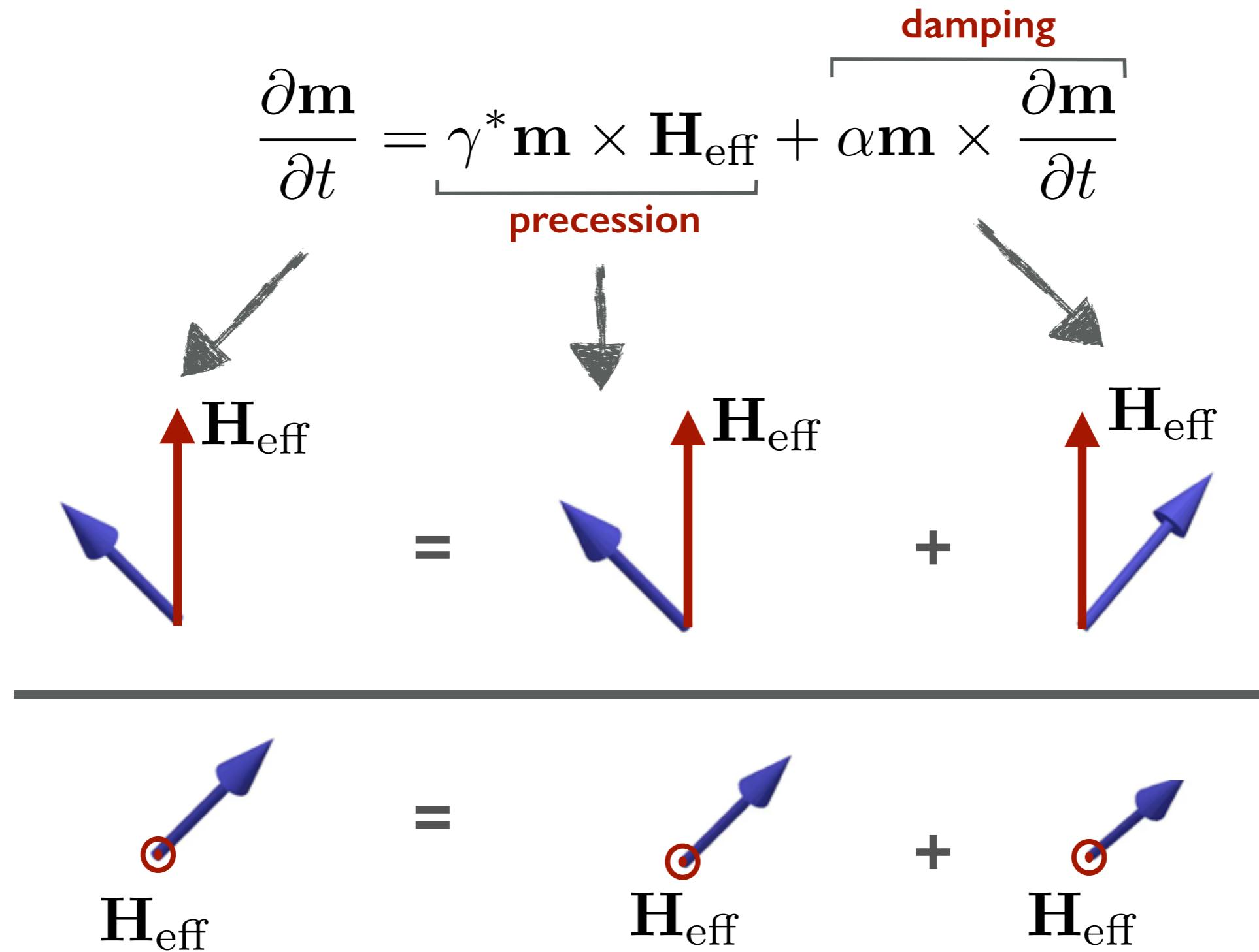
The diagram illustrates the LLG equation. At the top, the equation is shown as:
