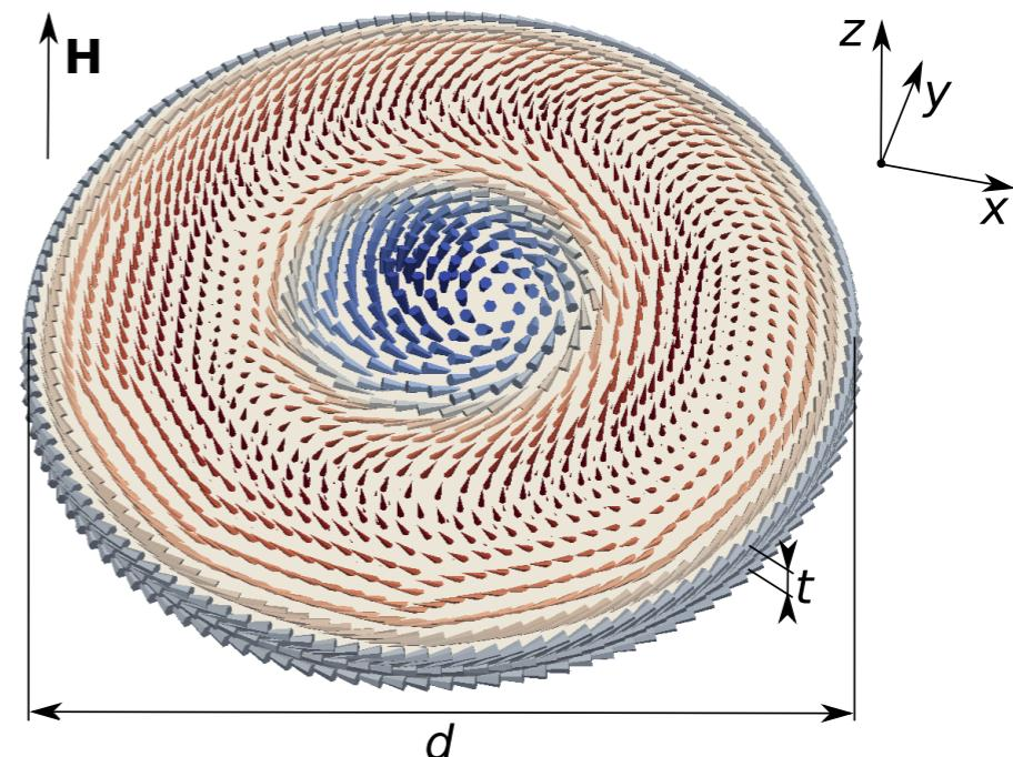
**Sample geometry and sample skyrmion ground state**
