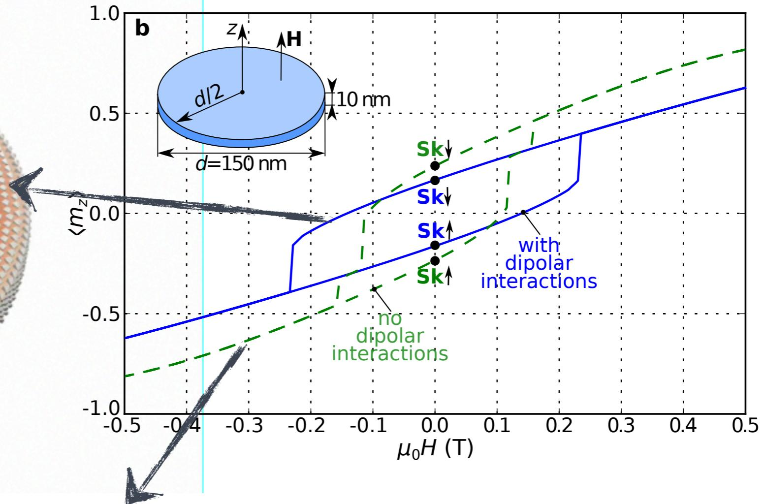
Hysteretic behaviour remains **in absence of** magnetocrystalline anisotropy and dipolar-based shape anisotropy, suggesting the existence of Dzyaloshinskii-Moriya based shape anisotropy.
